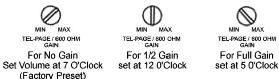
**NOTE:** This control works in conjunction with the master volume located on the front pane. If the master volume control is set at 0, then, regardless of how loud the 600 ohm/Tel-Page gain is set, the amp will not send an output to the speakers.
